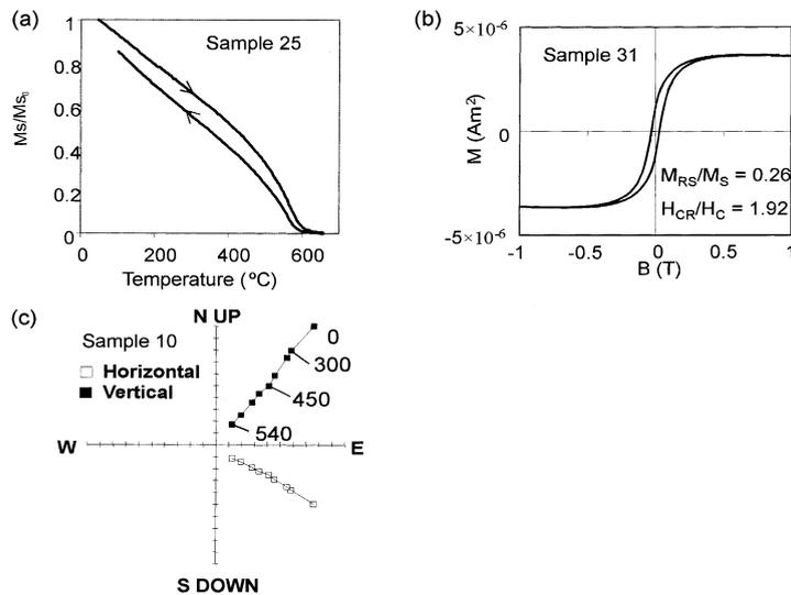
Fig. 2. Representative  $M_s(T)$  curve (a), hysteresis loop (b), and orthogonal vector plot (c) for Xitle lava samples, as derived from thermal demagnetisation data (temperature stages are provided in  $^{\circ}\text{C}$ ).
