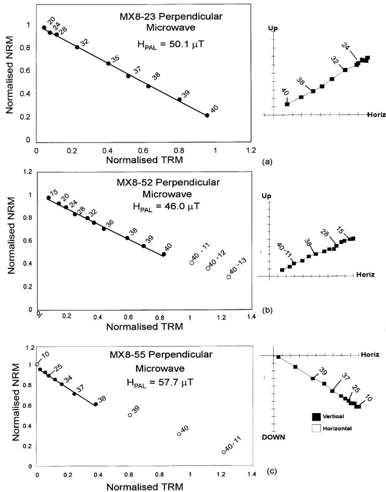
Fig. 5. Representative Arai and associated orthogonal vector plots for samples treated using the microwave Thellier method. Annotations are as for Fig. 4.
